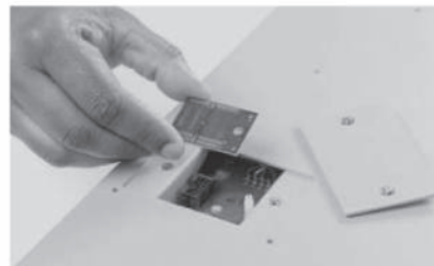
Figure 9. Installing the N7908A BBR hardware option on an APS power supply
